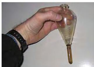
Picture 5. Water contamination test sample from ammonia chiller showing water/calcium chloride contamination of the ammonia close to 7%.
