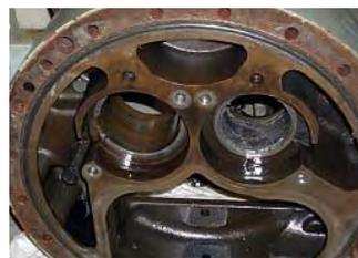
Picture 2: Slide bearing seizure on screw compressor due to lack of oil viscosity.
