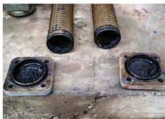
Picture 1: Compressor suction filters from an ammonia system contaminated with oil additives.
