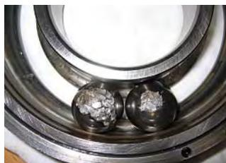
Picture 3. Broken ball bearing from screw compressor with water contamination of the oil.
