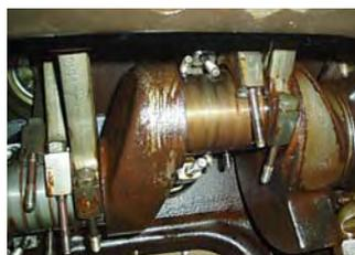
Picture 6. Crank shaft on ammonia compressor where the system is suffering from pollution with chlorine.
