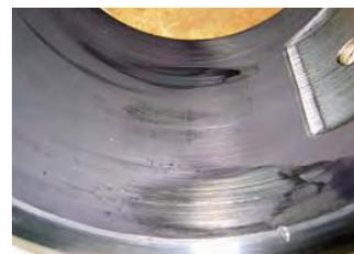
Picture 4. Slide bearing suitable for further use from same screw compressor with water contamination of the oil.
